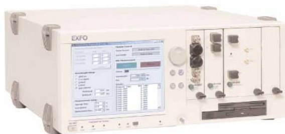
Figure 6. Test station comprising the IQS-505P platform, the IQS-2600B Tunable Laser Source, the IQS-5100B Polarization Scrambler and the IQS-3400B PDL/OL Meter
