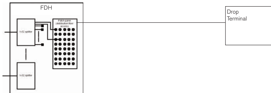
Figure 3. Fiber distribution hub (also called primary flexibility point or PFP), distribution fiber and drop terminal.
