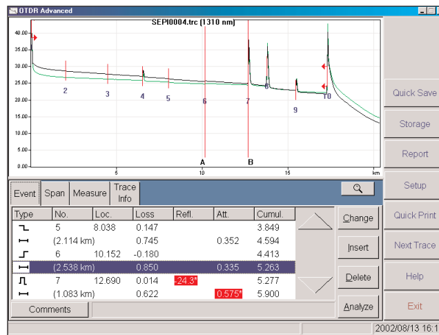
Figure 1: A screenshot of a typical OTDR measurement, displaying both the trace and its table of events
