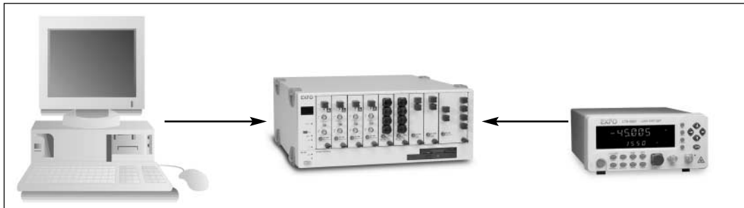
Figure 1. Typical GPIB Configuration
