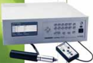
LSS-8000 Inchworm® Microdrive System
